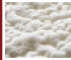
2" thick door tube injected with urethane insulation
